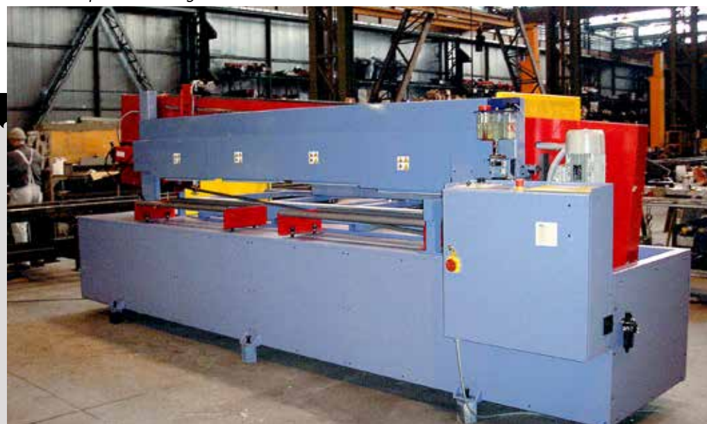
Taglio pannelli poliuretano 3.000 x 130 mm Polyurethane insulated panel cutting 3.000 x 130 mm
