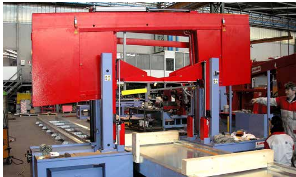
Taglio pannelli poliuretano in pacco 1.250 x 800 x 13.000 mm Insulated panel cutting in bundles 1.250 x 800 x 13.000 mm
