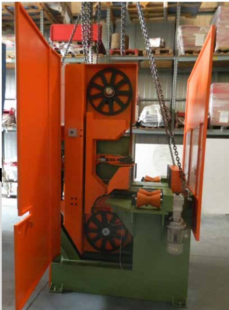
Taglio verticale Ø 420 mm Vertical cutting Ø 420 mm
